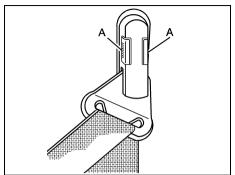
To move it up or down, squeeze the release buttons (A) together and move the height adjuster to the desired position.
